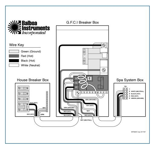
\* Actual wiring of GFCI will vary by manufacturer of GFCI. The GFCI shown is a Square D. Improper wiring of GFCI may result in permanent damage to spa system box. Repair / replacement of swim spa system box is not covered under warranty when damage results from improper wiring.
